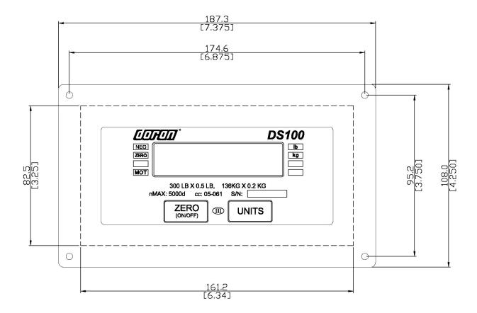
The cutout required for remote switch installation is 2.0" wide by 1.8" high. The minimum depth required for the main and remote display is  $1\frac{3}{4}$ " plus an additional 2.0" for the cable. The display is mounted by four #6 wood screws with a 90 degree countersink.
